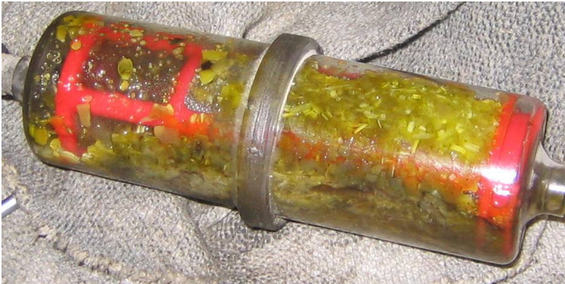
Figure 5-13 Inline pre filter which was partly blocked by small particles of solid fat, released from a small piece of zinc coated steel in the PPO tank
