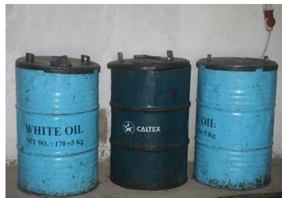
Figure 4-10 Oil drums for sedimentation (photo: Diligent Tanzania Ltd.)
