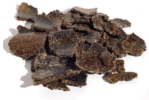
Figure 1-7 Pieces of presscake, pressed by a strainer press (photo Rural Biodiesel – Brazil)
