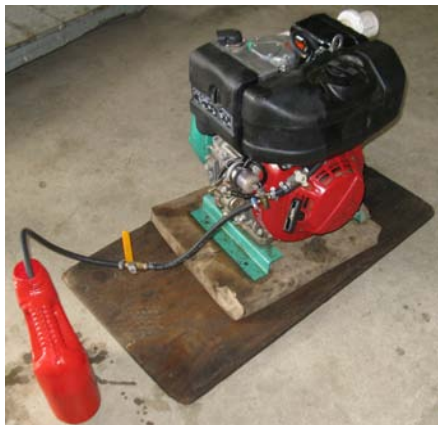
Figure 5-16 Two examples of converted engines. Left: Irrigation pump with Lombardini 15 LD 440 (1 cylinder 442ccm, 10.5hp) air cooled DI engine with manual start. Converted with a simple 2-tank system, Honduras October 2008 (Gota Verde Project). Right: Toyota Hilux 2,8D (3L). IDI engine. Converted by an ELSBETT 1-tank system, Honduras October 2008 (Gota Verde Project)
