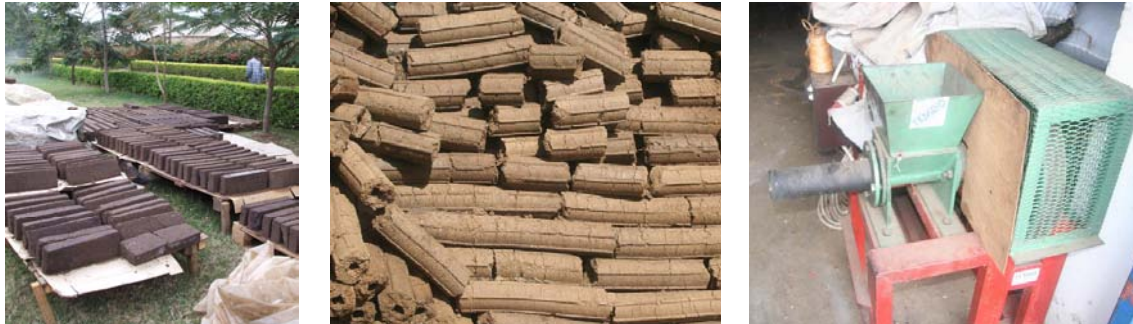
Figure 5-21 Presscake briquets and briquetting press (right) at Diligent Tanzania Ltd.
