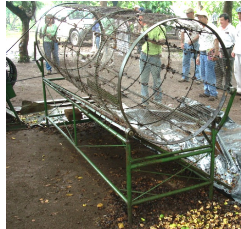
Figure 3-3 Sketch and photograph of a separator (used in the Gota Verde project, Honduras)
