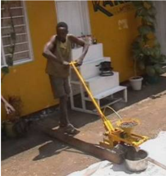
Figure 4-3 The Bielenberg ram press operated at Kakute Ltd., Tanzania [12]
