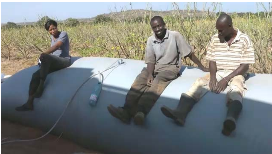
Figure 4-11 Pressure testing of a 12m 3 digester. The bottle provides a protection against over pressure.
