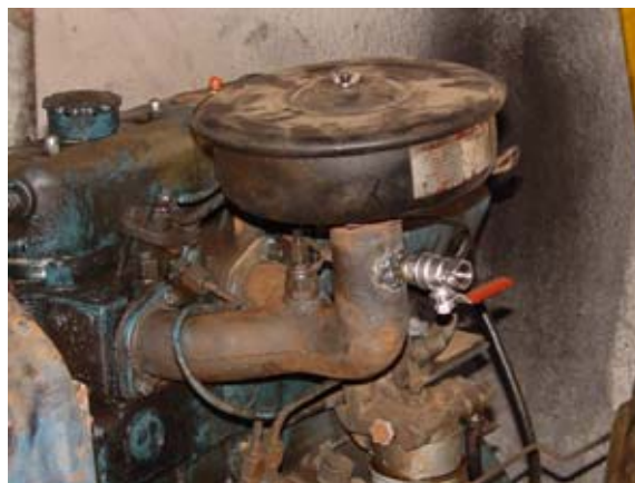
Figure 7-18 The valve connection to the air inlet
