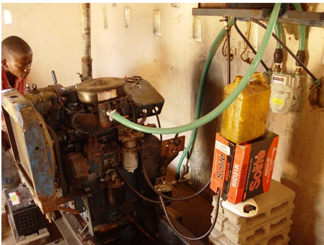
Figure 7-19 The gas system connected to the diesel engine, in a test setup.
