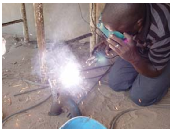
Figure 7-16 Welding the thread to the inlet
