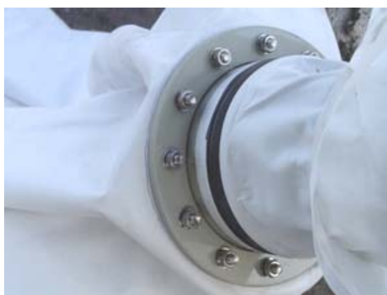
Figure 4-1 PVC Bag inlet flange
