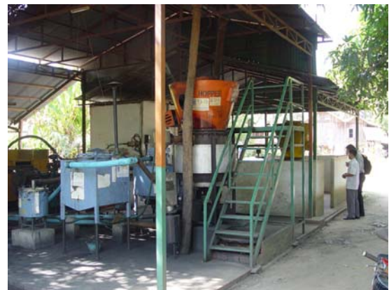
Figure 1: A 22 kW gasifier used for village electrification in Cambodia
