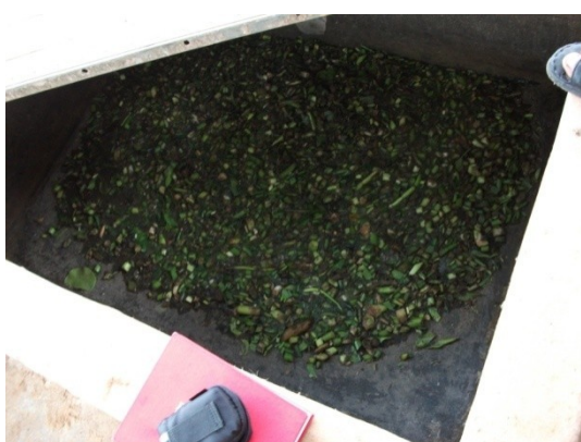
Figure 21: Chopped E. Crassipes as feed stock in the biogas inlet tank, Songhaï Centre, Porto Novo
