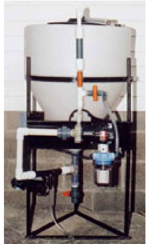
Figure 12: 300-litre biodiesel processor (Source: Biodieseltgear.com ).
