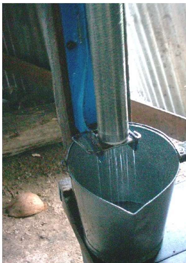
Figure 11: DME press with oil produced (Source: SOPAC).
