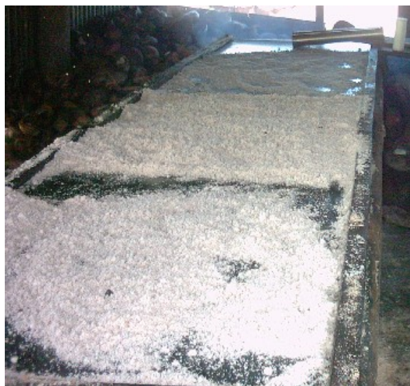
Figure 10: Grated coconut drying for DME processing (Source: SOPAC).
