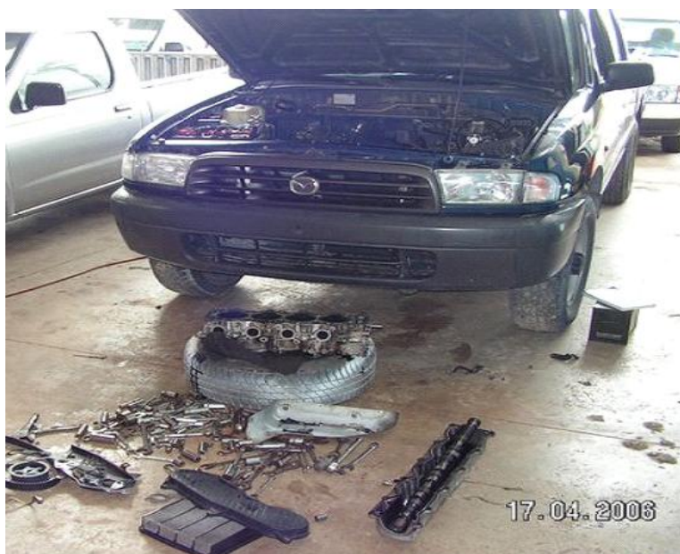
Figure 20: RMI truck that ran on coconut oil for three years showed signs of increased maintenance requirements (Source: Fürstenwerth).
