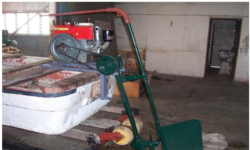
Figure 24: Boat powered with indirect injection engine from China run on coconut oil by National Fisheries College (Source: Carr, Walton, Rigby, National Fisheries College, Papua New Guinea).
