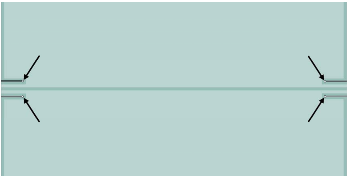
Figure 11 Top view of digester bag, with spots requiring reinforcements
