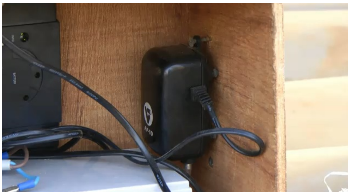
Figure 20 A small aquarium pump supplying air to a digester. The pump (4W) is fed with a small PV system
