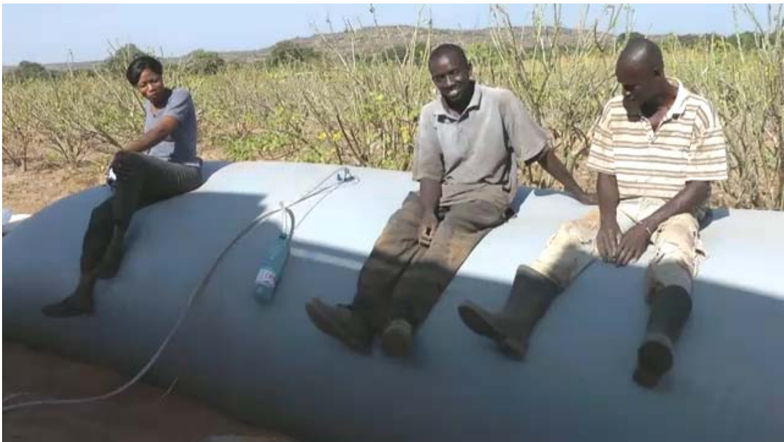
Figure 18 Pressure testing in progress. The bottle provides a protection against over pressure.
