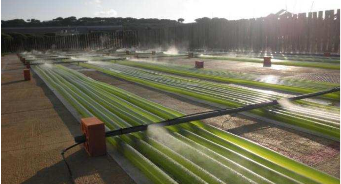
Figure 22: Closed tubular photobioreactor, Wageningen University
