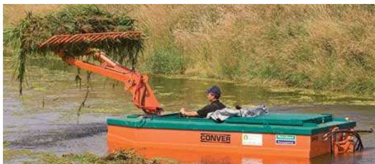
Figure 15: Mowing boat with rakes attached for removing typha and reed stems
