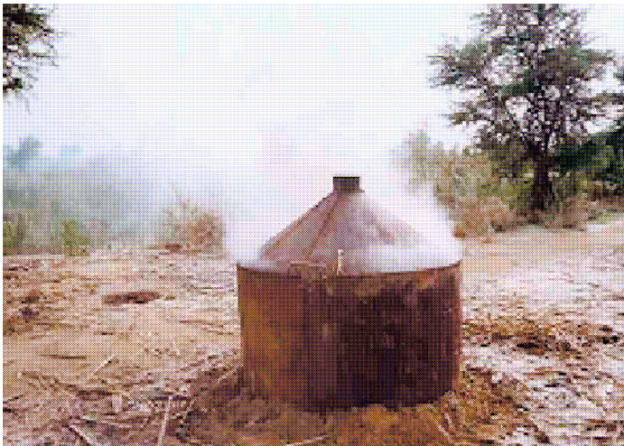
Figure 17: PERACOD Charcoal reactor '3 fûts', Senegal
