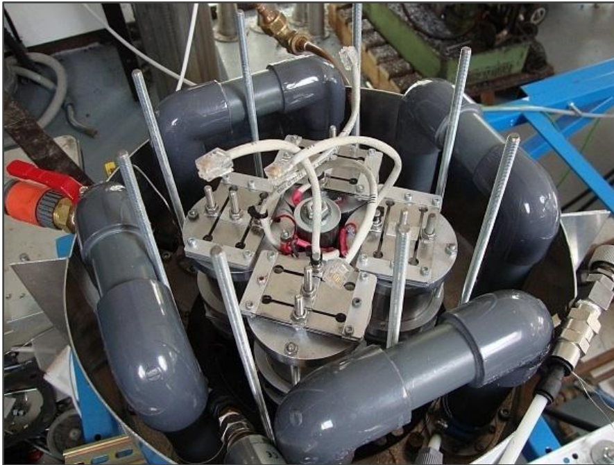
Figure 3.2: A thermo-acoustic generator with 4 linear alternators in the middle
