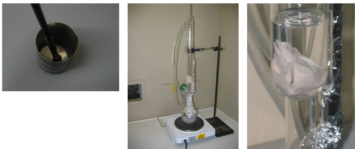
Figure E-2 equipment used for soxhlet extraction from left to right: mortar and pestle to grind samples before extraction, soxhlet setup, filter paper instead of extraction thimble.
