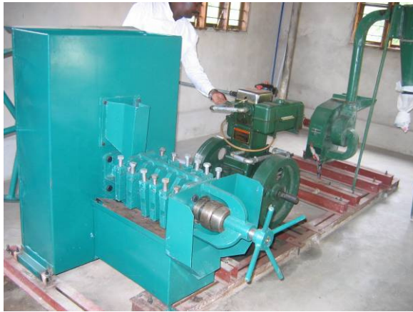
Figure 7-1 Left hand picture: A TaTEDO test MFP near Dar es Salaam with from left to right a Sayari screw press, Lister engine and a maize mill. Between the engine and the maize mill normally a generator is fitted like the blue one shown in the right hand picture that was taken in Engaruka.
