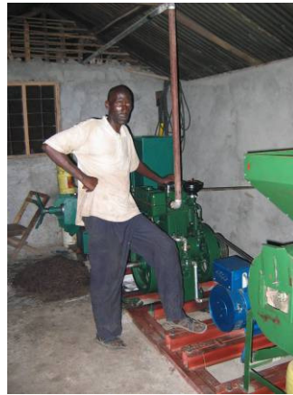
Figure 7-1 Left hand picture: A TaTEDO test MFP near Dar es Salaam with from left to right a Sayari screw press, Lister engine and a maize mill. Between the engine and the maize mill normally a generator is fitted like the blue one shown in the right hand picture that was taken in Engaruka.
