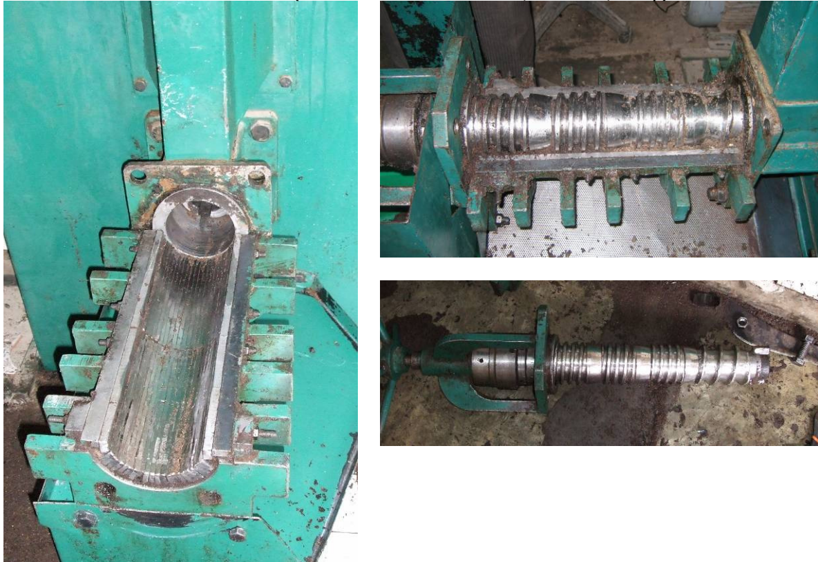
Figure F-1 Detailed views of the Sayari expeller. Left: the press cage made from separate lining bars. Right top: worm positioned in the bottom part of the cage. Right bottom: separate worm with clear distinction between cones and transport screw. The wheel on the left is for manual adjustment of the outlet restriction.
