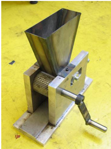
Figure 4-2 Hand powered de-huller designed together with Gerard van Hout from the workshop at Mechanical engineering.
