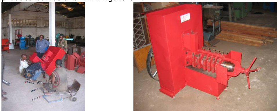
Figure F-2 Assembly of Sayari expeller at Intermech workshop and final product.
